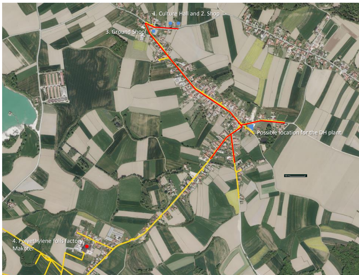
Figure 1: Cven settlement consumers and the DH grid in red line (yellow lines show the natural gas grid), location of the possible plant
