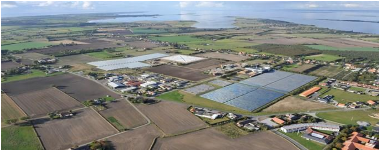
Figure 7: Marstal solar district heating and seasonal pit heat storage (Source: www.solarmarstal.dk )
