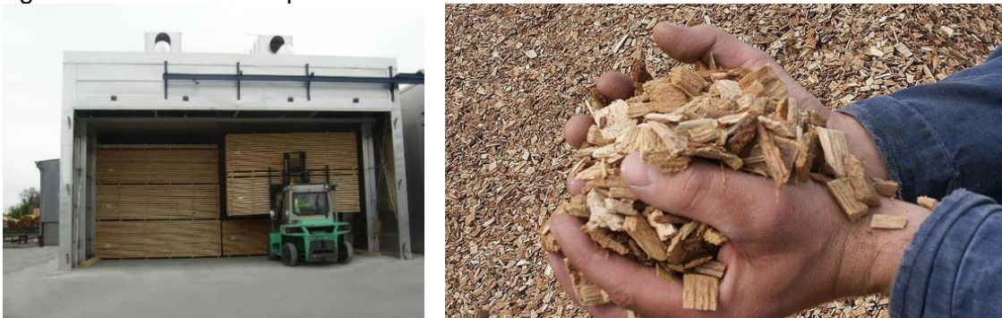
Figure 21: Drying chambers for wood floor production are heated with the district heating in Güssing; Wood chips as input material for heat production in the boilers (Source: Güssinger Fernwärme GmbH)
