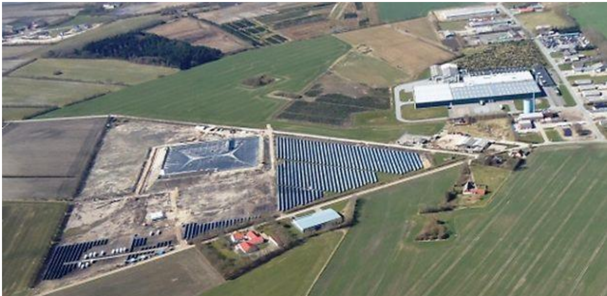
Figure 4: The seasonal pit storage and the solar field under establishment. To the right is the existing 10,000 m 2 and at left and front is seen the area where the new solar panels installed together with the seasonal pit storage, picture by Gram Fjernvarme
