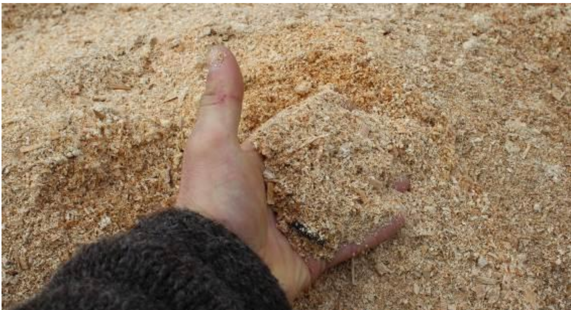
Figure 18: Saw dust that is used as a fuel for the CHP and heating plant
