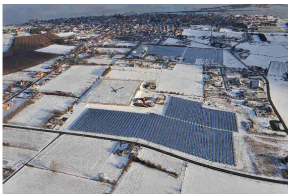
Solar district heating and pit thermal energy storage (seasonal) in Marstal, Denmark
