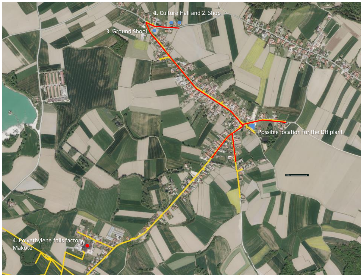
Figure 6: Cven settlement consumers and the DH grid (red line), location of the possible plant
